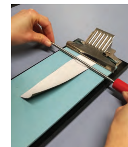
Varnishing with a spiral blade
